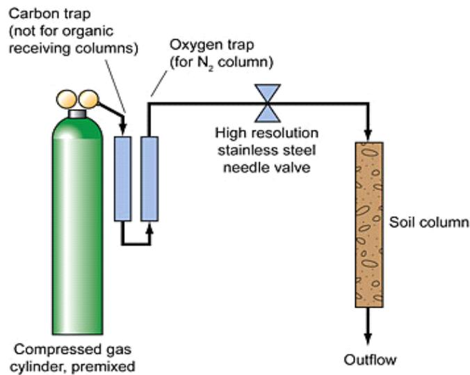
Schematic of the treatment system used for laboratory studies.
